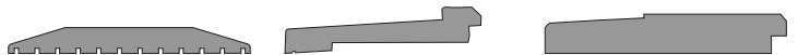
10007 Pivot door solid wood sill 3/4" thick 10008 Inswing solid wood sill 1-5/8" thick at dam 10009 Outswing solid wood sill 1-5/8" thick at dam
