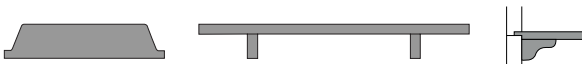
9526 For exterior 1-3/4" and 2-1/4" dutch doors with either dutch and dado OR dutch and rabbet 3/4" thick, 7-1/8" deep, brackets predrilled. Make sure to specify door thickness and type of dutch cut (screws not included - requires four 1-1/4" long #6 wood screws).
