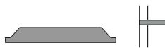
9525 For interior 1-3/8" or 1-3/4" dutch doors with straight dutch cut 3/4" thick, 4-3/8" or 4-3/4" deep. Make sure to specify door thickness
